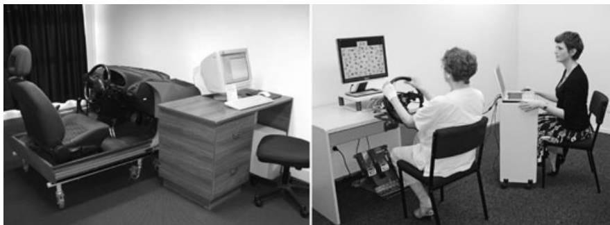
Figure 1. (A) Modified car body used to run SMCTests at the Driving and Vehicle Assessment Service site. Test stimuli were projected onto a white wall in front of the apparatus. (B) Portable apparatus used at the other two sites. Stimuli for the portable version were presented on a computer monitor.
