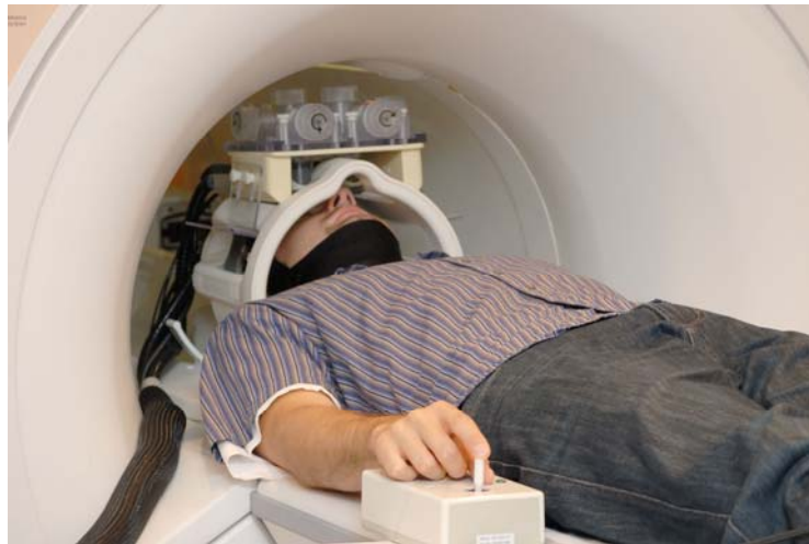
Figure 2. A participant, just before fully entering the scanner, with the MagLink 64-ch. EEG cap, the Avotec binocular video display & eye camera, and the 2-D joystick (all MR-compatible).
