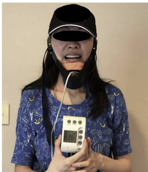
Fig 1 A compact dynamometer secured under the chin and to the head using custom-made, adjustable head straps was used for measuring jaw-opening strength. Maximum force generated at each trial was displayed on the monitor.
